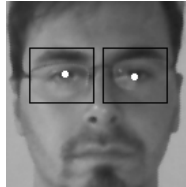
Fig. 3. Customer's face detected by the face re-identification framework. The face is considered for further processing only if both eyes are detected. Eyes position are used to remove scale and rotation variabilities before feature extraction.
