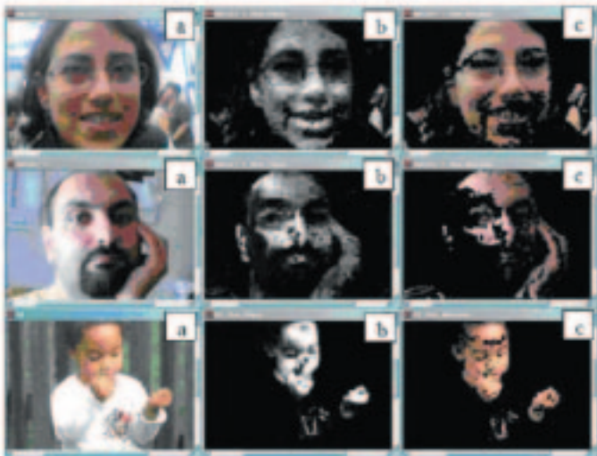
Figure 1: Skin recognition examples on RGB images: a) original images acquired by Nokia 7650 phone (first and second row) with VGA sensor and compressed in jpeg format; b) probabilistic threshold output; c) simplest threshold method output. Third rows image (a) is a standard test image.
