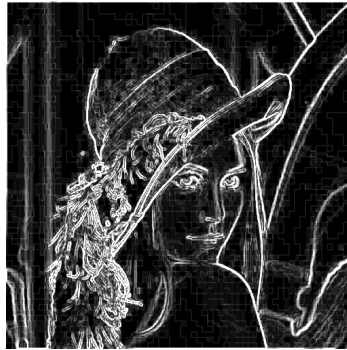
Fig.6: Effect of the Sobel filter (3x3 kernel size) applied to the Lena image.
