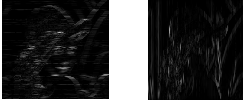
Fig.7: 30 taps directional HPF applied to the Lena image. Borders are not considered (thus the vertical size in the left image and the horizontal size in the right images are less than the original size).
